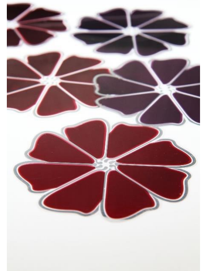
Reverse offset printing (ROP) printing and flexible OPV cells.
