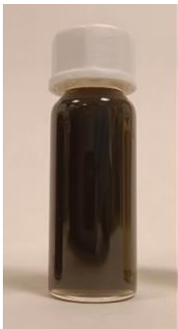
Left: graphene ink in cyrene. Centre: representative TEM micrograph of a graphene flake. Right: spray-coated conductive graphene electrode.
