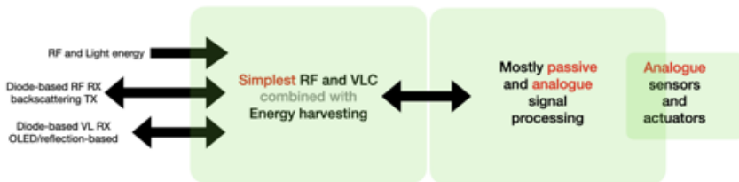
All-printed node architecture
