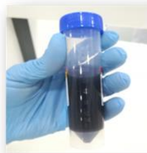
Graphene dispersion in 2-Propanol
