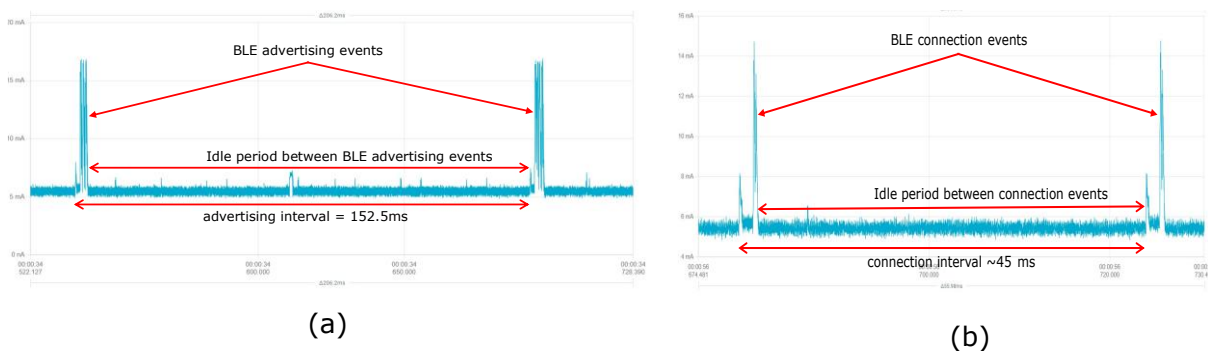
Figure 3.3.6. Illustration of the current profile of a single: (a) BLE advertising interval, (b) BLE connection interval.
