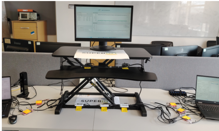
Figure 44. Actual experimental IoT network energy measurement setup.
