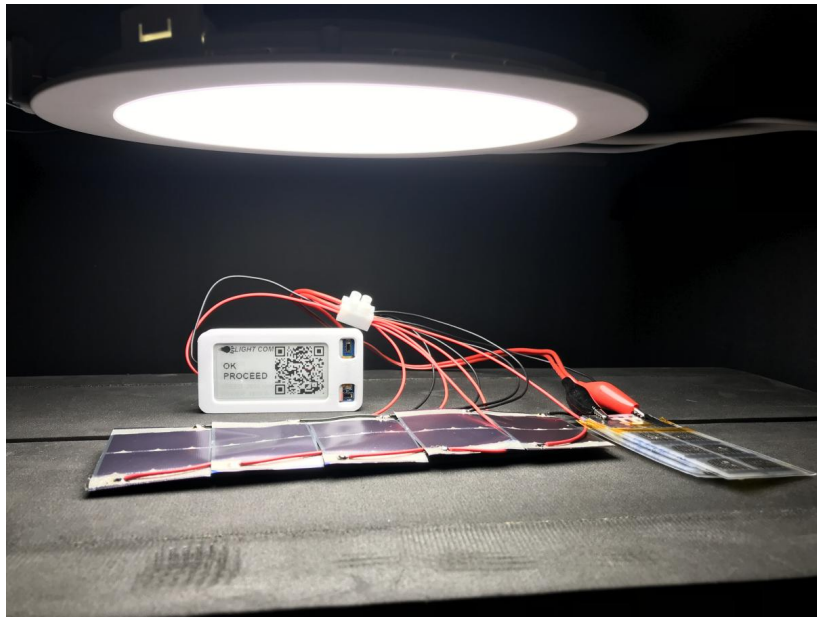
Figure 29. The hybrid SUPERIOT node combines printed electronics (PE) and Si-based technologies.
