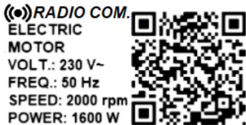
Figure 16. Information and data for controlling the industrial material flow: electric motor product nameplate – data received via RF BLE downlink.
