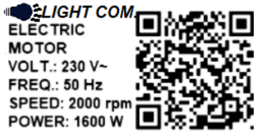
Figure 12. Information and data for controlling the industrial material flow: electric motor product nameplate – data received via VLC downlink.
