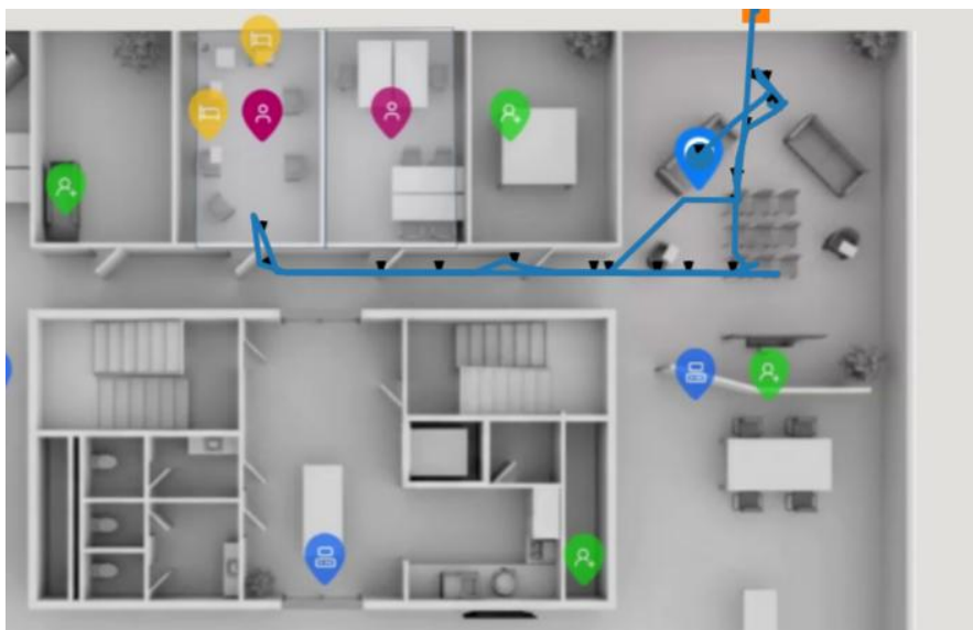
Figure 23. Bluetooth Channel Sounding real-time position data during scenario 1 of demonstrator 2.
