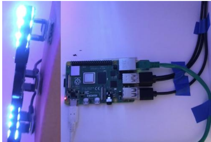
Figure 15. Access Point for the printed IoT node – RGB lamps on the left and Raspberry Pi SBC on the right.
