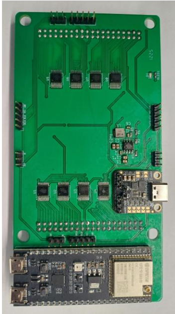
Figure 3. Control board with 8 shift registers totalling 64 bits for the PIN diode-based cells.
