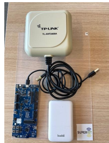
Figure 10. BLE channel sounding anchor (directional antenna, Nordic DK, and power bank).
