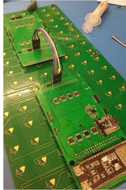
Figure 4. Two control boards forming a series of 16 shift registers to control two tiles.
